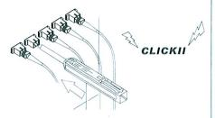
Be careful not to slant the One-Click Cleaner SC while inserting into the adapter.
