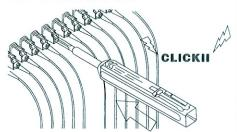
Be careful not to slant the One–Click Cleaner MU/LC while inserting into the adapter. Do not overly exert force during insertion as this may cause damage to both the connector and the One–Click Cleaner MU/LC. If pushing Outer Shell is inhibited,remove One–Click Cleaner MU/LC form adapter and ensure that there is no sizeable debris inhibiting the cleaning process.
