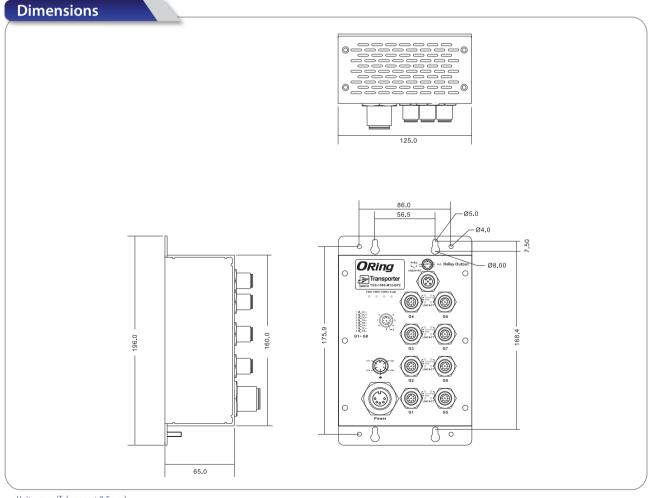
Unit =mm (Tolerance ±0.5mm)
